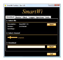
The main function of the Toolbox is to download a new firmware to your SmartWi system. You must first connect the SmartWi Master box to your PC, via a standard USB cable.
